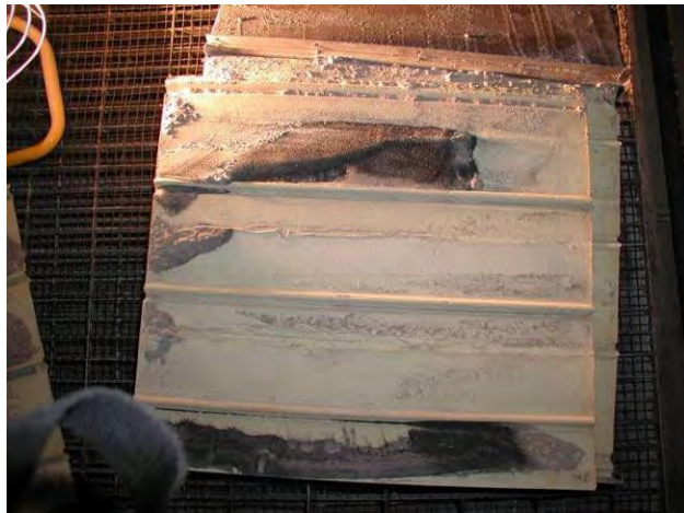
Plate Catalyst With Accumulated Unburned Carbon
