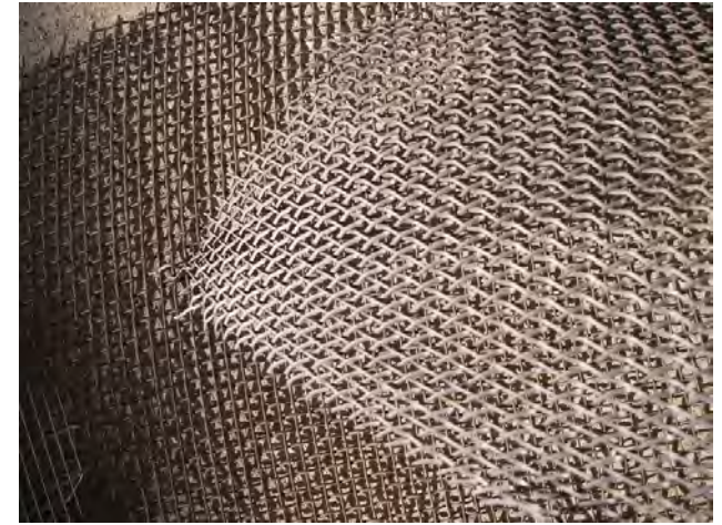
Coated & Non-Coated Screens Failed (High Velocity)
