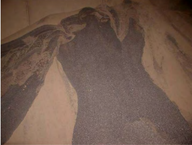
Reactor Accumulation of Unburned Carbon
